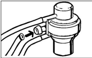
Remove hose from connection port B. (This hose runs between the canister control valve and the carbon canister.) Do NOT plug the hose for the remainder of the test procedure. Be sure to reconnect the hose after testing and servicing is completed!
