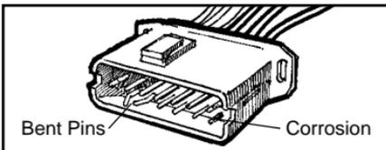
Problems with connectors are common in the engine control system. Inspect carefully. Note that some connectors use a special grease on the contacts to prevent corrosion. Do
