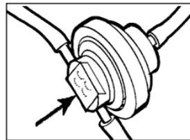
Cover the atmospheric vent holes with a piece of tape. Be sure to remove the tape after testing and servicing is completed!
