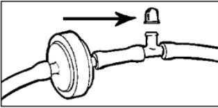
There is a tee with a restrictor in the Thermactor Vacuum control line. The restrictor must be uncapped during the test. Replace the cap after testing. Refer to drawing for location of restrictor on the TAD vacuum line (4.2L engines) or the TAB vacuum line (5.8L engines).
