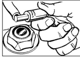
Remove PCV valve from breather cap on valve cover. Be sure to replace PCV valve after testing and servicing is completed!
