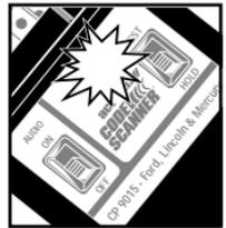
**NOTE:** If a fault is recreated this way, a service code will be stored in computer memory. Be sure to erase this code from memory after making all repairs. Refer to Section 4 (Self-Test Part 5: Erasing "Continuous Memory" codes).
