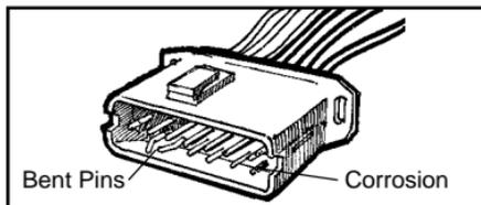
Problems with connectors are common in the engine control system. Inspect carefully. Note that some connectors use a special grease on the contacts to prevent corrosion. Do not wipe off! Obtain extra grease, if needed, from your vehicle dealer. It is a special type for this purpose.
