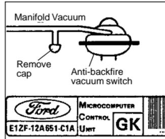
Remove the cap from the anti-backfire vacuum switch tee during testing. The switch is located behind the MCU module. Be sure to replace the cap after testing and servicing is complete!
