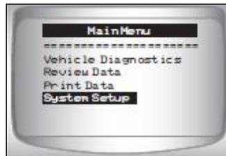
3. In the **System Setup** menu, arrow down to **Program Mode** and press **ENTER**.
