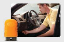
2. Plug U-Scan® into vehicle port usually found underneath steering column.
