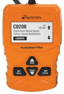
Patent No. Des. 6,701,233 Patent No. Des. 6,928,349 Diagnostic Trouble Codes (DTC's) and descriptions are just a start of the tasks it can handle. PocketScan Plus also provides freeze frame data, permanent DTCs, VIN info and performs the important task of Inspection Maintenance (I/M) readiness testing by displaying the I/M readiness monitor status.
